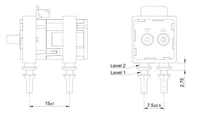
Drill hole, level 2: 3.5 mm Drill hole, level 1: 3.0 mm
